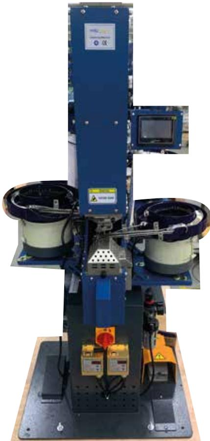
WA8811 is a full automatic machine for special press-fasteners and eyelets that can be assembled on textiles, leather, handbags, cardboard and plastic. It makes the punch hole automatically and then assemble the for ex eyelet.
