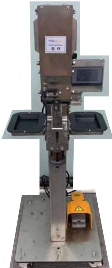
WA20 is a semi automatic machine for Press-fasteners, Jeansbuttons, rivets and eyelets that can be assembled on textiles, leather, handbags, cardboard and plastic.
