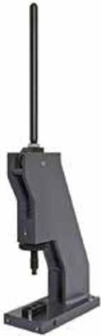
Manual assembling machine of toggle joint type for press-fasteners, jeans-buttons, rivets etc.
