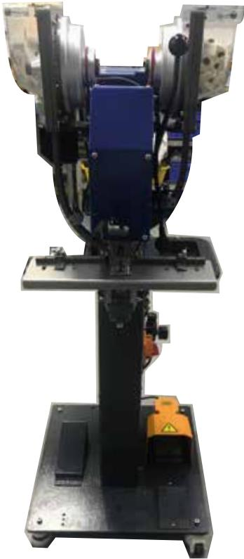
WA95 is a full automatic machine for Press-fasteners, Jeansbuttons and rivets.that can be assembled on textiles, leather, handbags, cardboard and plastic.
